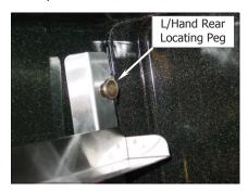
b. Locate the top front of the rack over the locating peg at the top front LH side of the oven.
